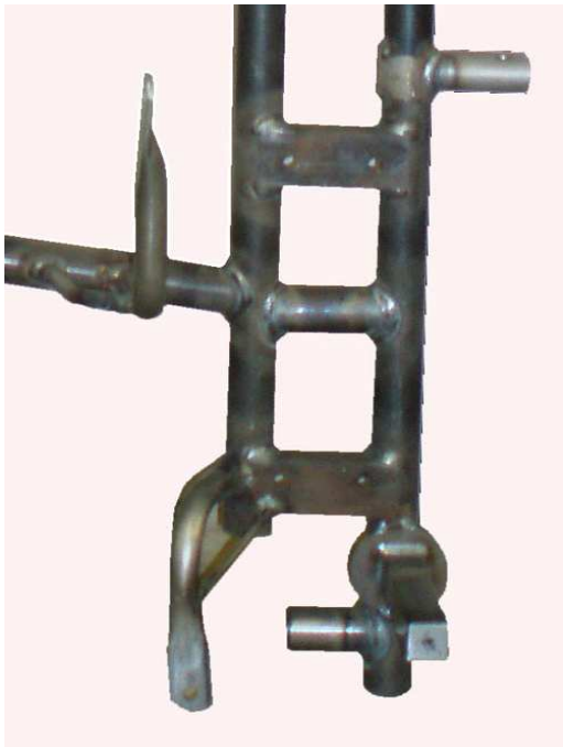
Photo from above of the frame with the section of the engine mount
