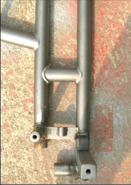
Photo from above of the frame with the section of the engine mount
