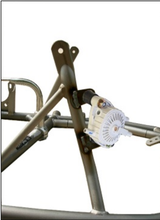
Photo of the frame with the section of the support for the fuel pump (fuel pump mounted)
