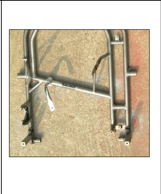
Photo from above of the frame with the section of the two supports for the RTPS (Rear Tire Protection System)
