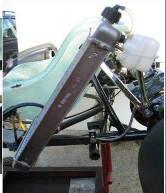
Foto of the frame from the side with the section of the supports for the radiator (radiator mounted)
