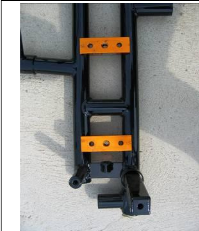
Photo from above of the frame with the section of the engine mount
