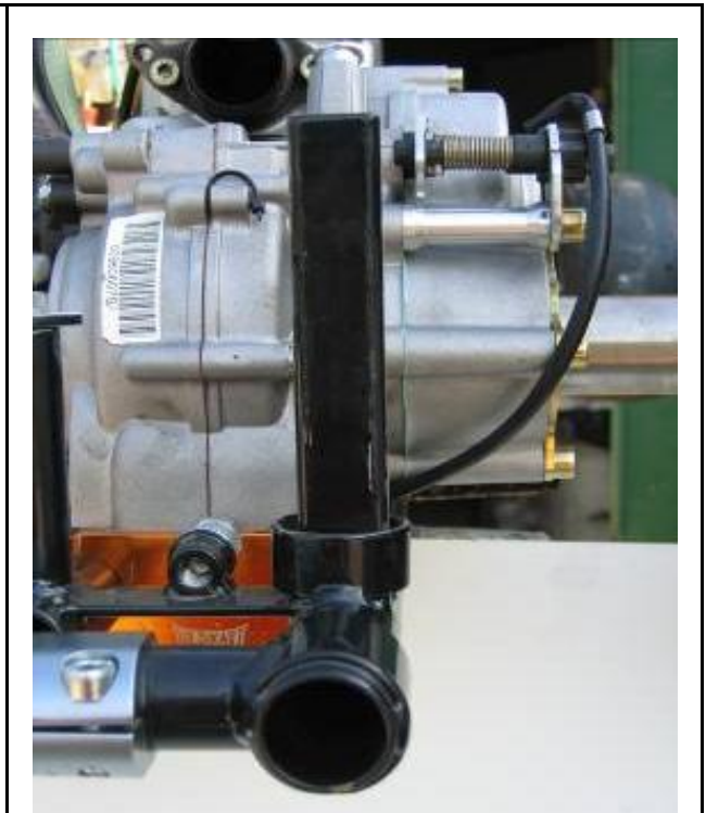
Photo of the frame from the back with the section of the support for the RTPS (Rear Tire Protection System)
