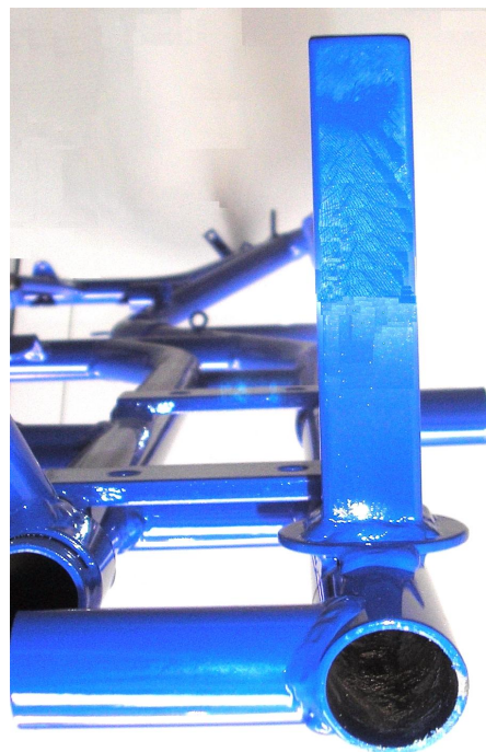
Foto of the frame from the back with the section of the support for the RTPS (Rear Tire Protection System)
