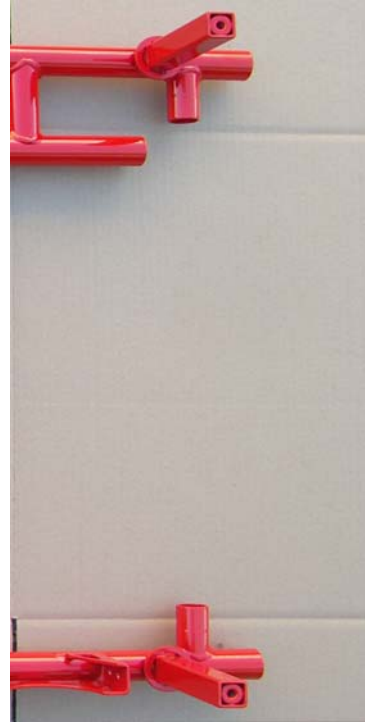
Photo from above of the frame with the section of the two supports for the RTPS (Rear Tire Protection System)
