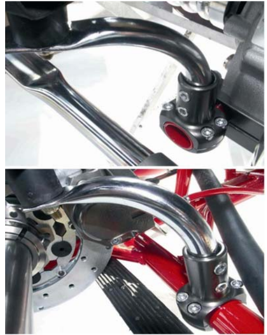
Photo from above of the frame with the section of the two supports for the exhaust system
