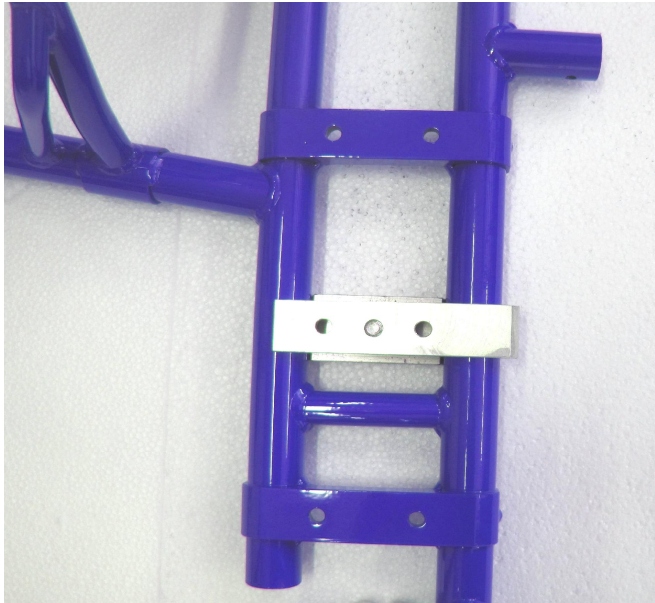
Foto from above of the frame with the section of the engine mount
