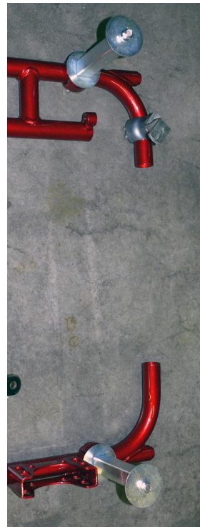
Photo from above of the frame with the section of the two supports for the RTPS (Rear Tire Protection System)
