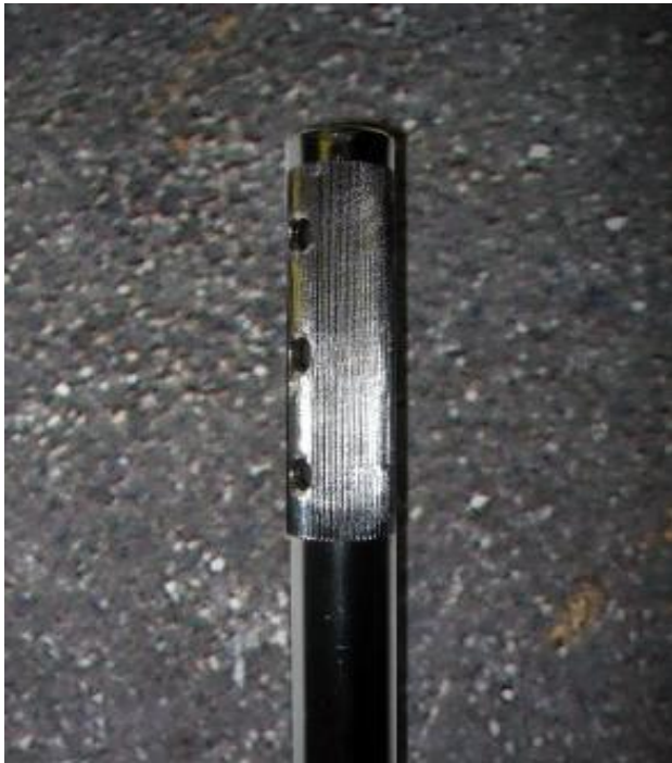
Photo from the steering column with the section with the knurling for the steering wheel hub (knurling according to DIN 82 - RAA1).
