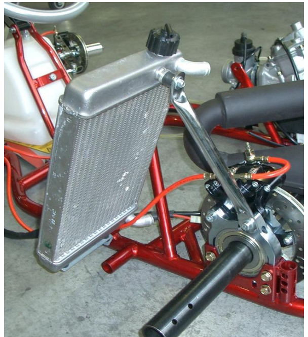
Photo of the frame from the side with the section of the supports for the radiator (radiator mounted)
