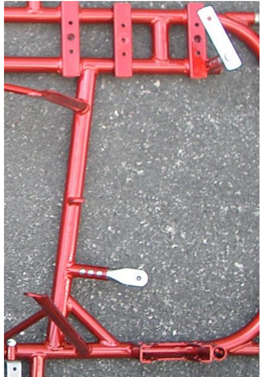
Photo from above of the frame with the section of the two supports for the exhaust system
