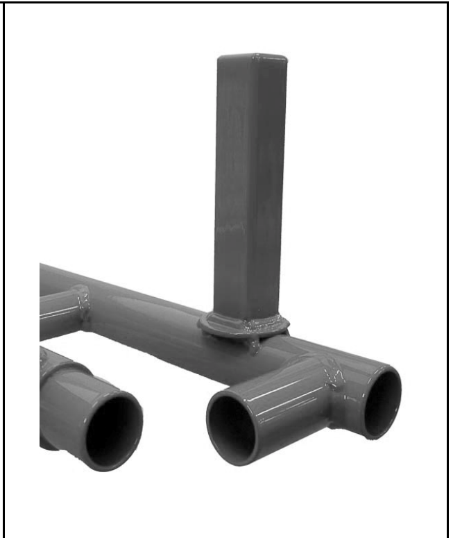
Foto of the frame from the back with the section of the support for the RTPS (Rear Tire Protection System)
