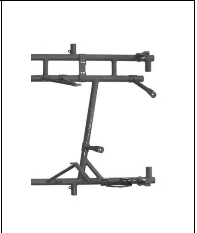
Foto from above of the frame with the section of the two supports for the RTPS (Rear Tire Protection System)
