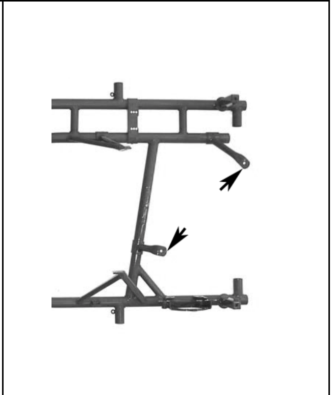
Foto from above of the frame with the section of the two supports for the exhaust system
