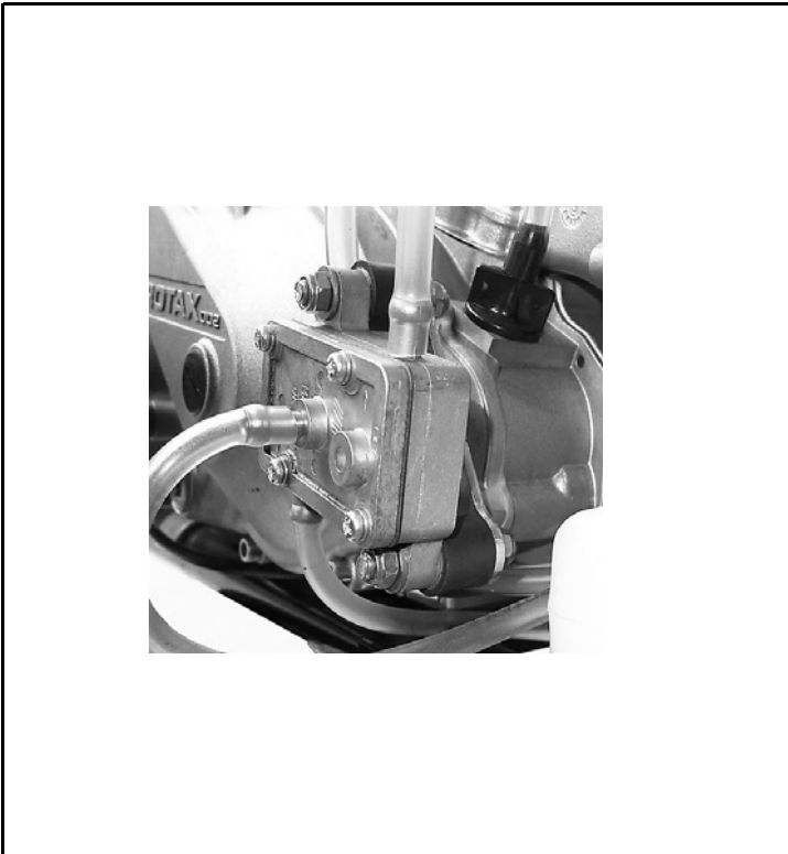
Foto of the frame with the section of the support for the fuel pump (fuel pump mounted)
