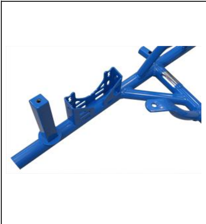
Photo of the frame from the side with the section of the support for the RTPS (Rear Tire Protection System)
