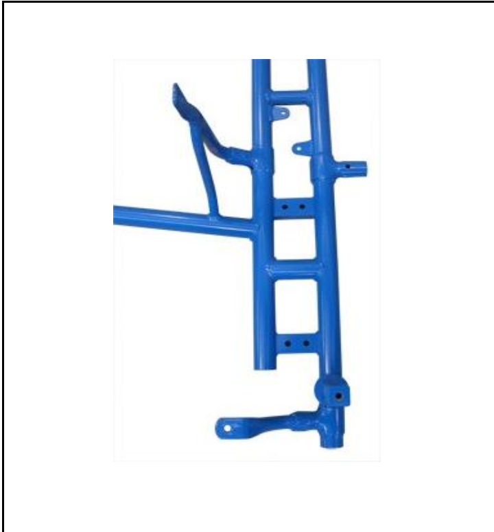
Photo from above of the frame with the section of the engine mount
