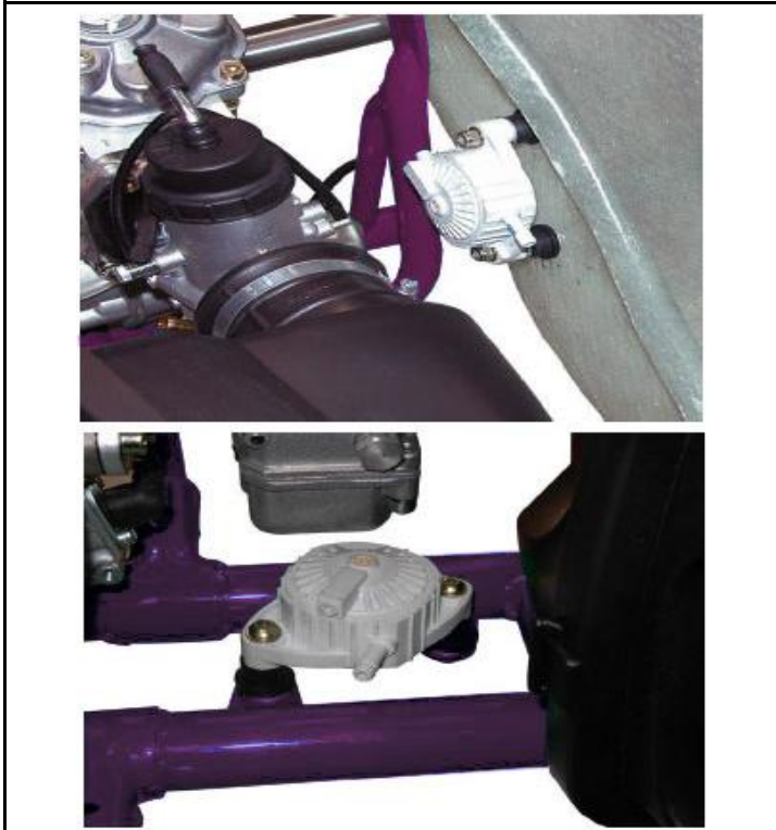
Photo of the frame with the section of the support for the fuel pump (fuel pump mounted)
