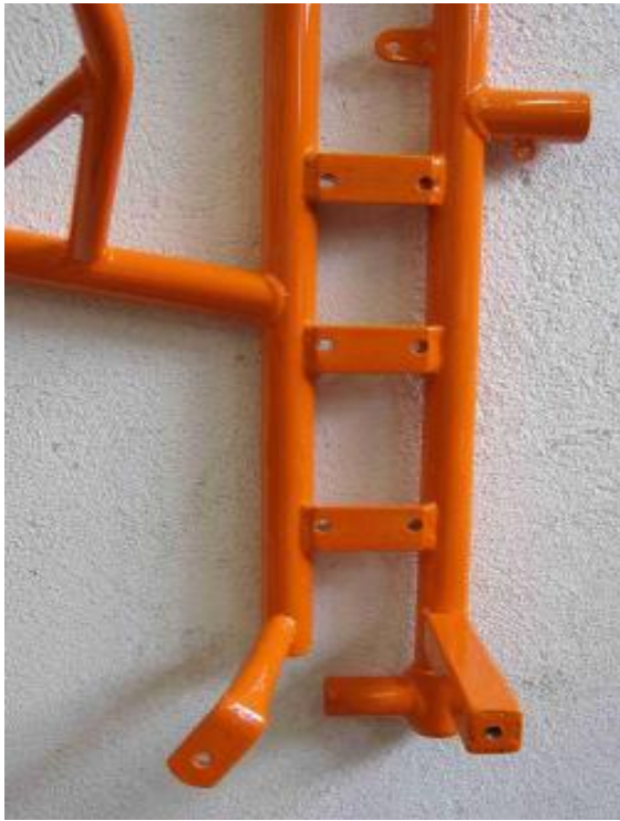
Foto from above of the frame with the section of the engine mount
