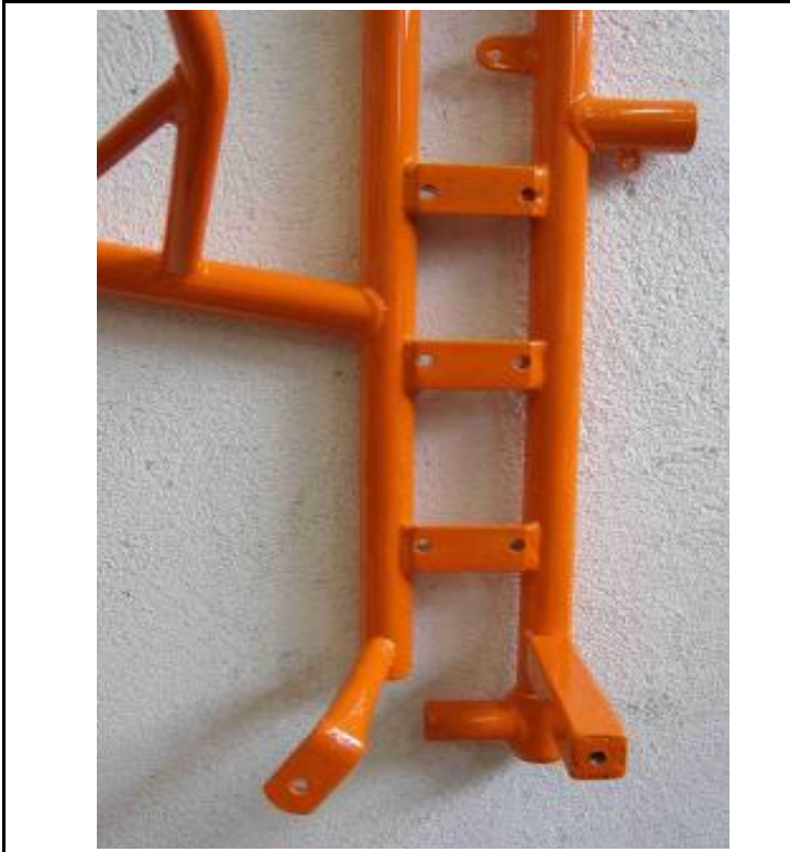
Foto from above of the frame with the section of the engine mount
