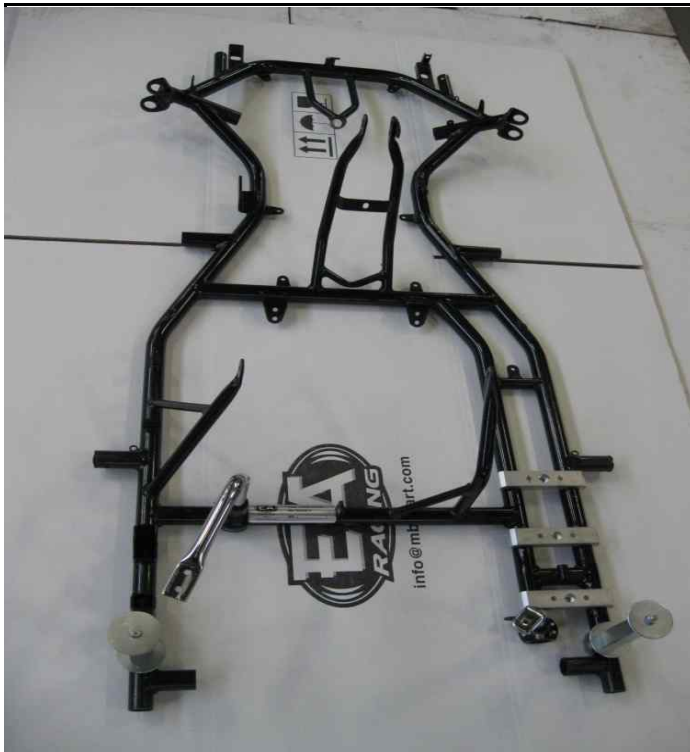
Photo from above of the frame (without any monted part)
