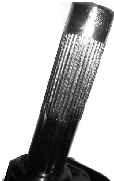
Foto from the steering column with the section with the knurling for the steering wheel hub (knurling according to DIN 82 - RAA1).
