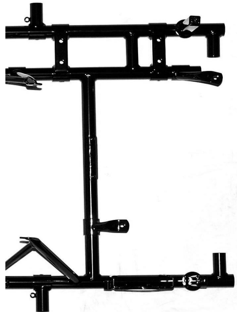
Foto from above of the frame with the section of the two supports for the RTPS (Rear Tire Protection System)
