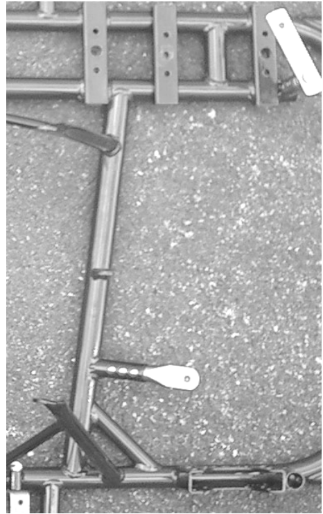
Photo from above of the frame with the section of the two supports for the exhaust system
