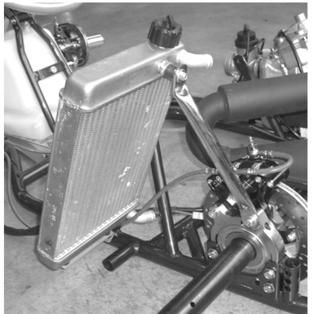
Foto of the frame from the side with the section of the supports for the radiator (radiator mounted)
