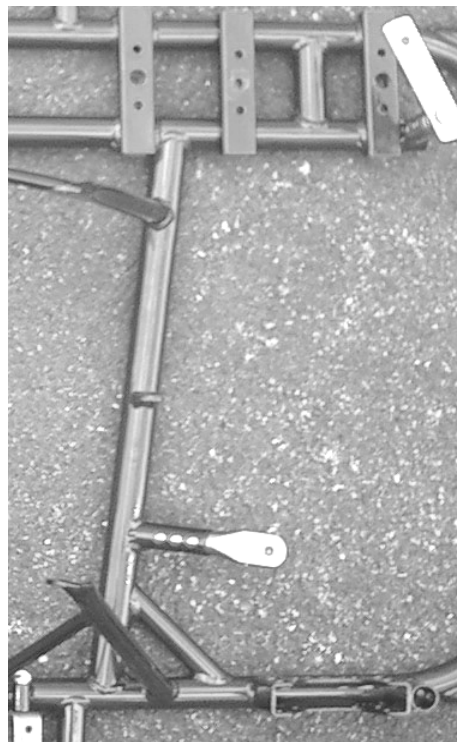
Photo from above of the frame with the section of the two supports for the exhaust system
