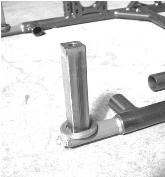
Photo from the steering column with the section with the knurling for the steering wheel hub (knurling according to DIN 82 - RAA1).
